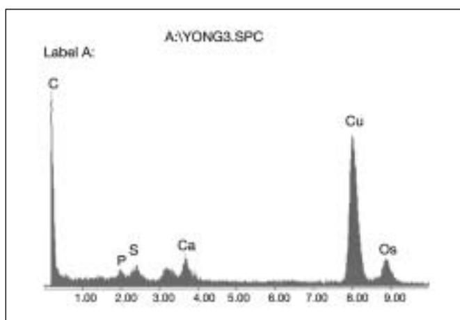
**Fig. 3** - EDX showing peaks of calcium and phosphorus in explanted IOL 1.
