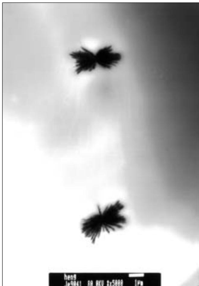
Fig. 2 - Transmission electron micrograph of the opacities (x 5000) in the explanted IOLs.
